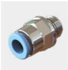
6.0mm OD to 1/8" BSPP Male Thread E-F-220039
