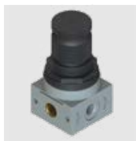
Relieving - 1/8" BSPP Female Thread 0 to 4 bar E-R-200005
