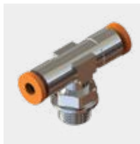
4.0mm OD to 1/8" BSPP Male Thread E-F-170778
