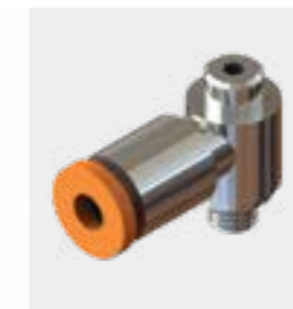
4.0mm OD to M5 x 0.8 Male Thread E-F-170755
