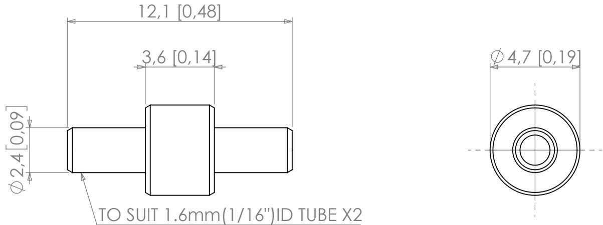
NOTE: PART CAN BE UTILISED IN EITHER FLOW DIRECTION
